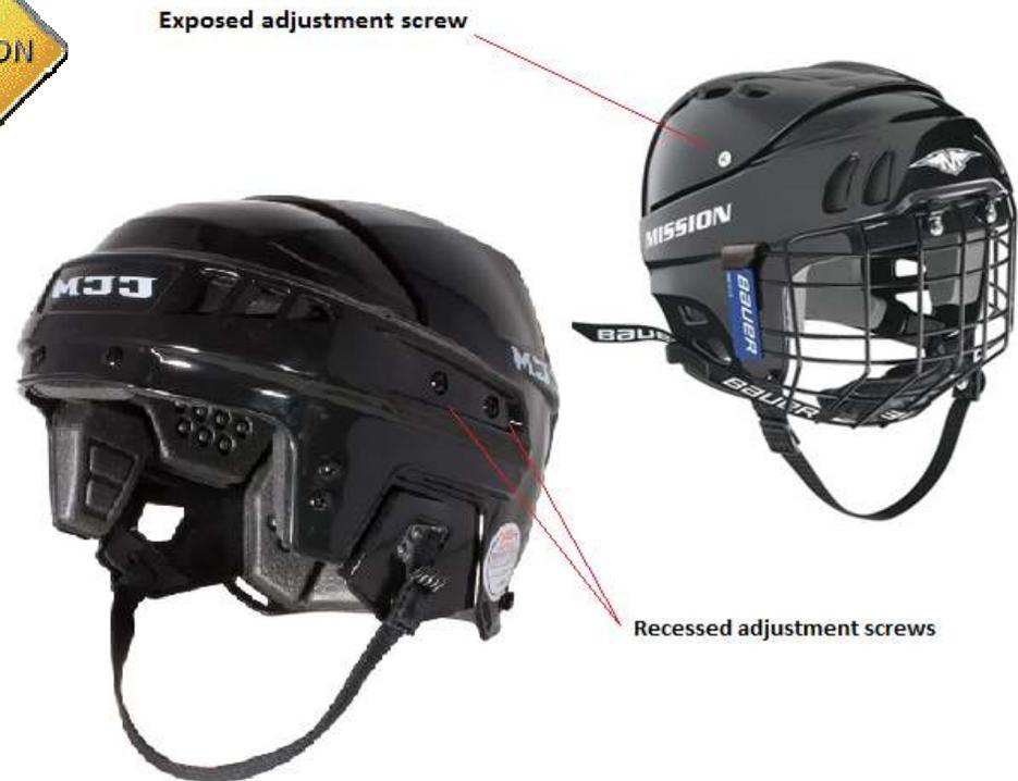
Often a washer, bonded to the helmet with epoxy, can be placed beneath the screw to strengthen the cracked area. But if the crack continues to grow, the helmet should not be used, especially in Div 2 and 3.
